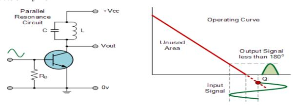
Due to its heavy audio distortion, class C amplifiers are commonly used in high frequency sine wave oscillators and certain types of radio frequency amplifiers, where the pulses of current produced at the amplifiers output can be converted to complete sine waves of a particular frequency by the use of LC resonant circuits in its collector circuit.
