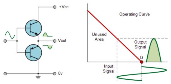
When the input signal goes positive, the positive biased transistor conducts while the negative transistor is switched "OFF". Likewise, when the input signal goes negative, the positive transistor switches "OFF" while the negative biased transistor turns "ON" and conducts the negative portion of the signal. Thus the transistor conducts only half of the time, either on positive or negative half cycle of the input signal.
