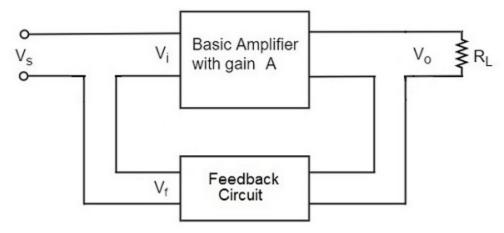
As the feedback circuit is connected in series with the output and the input as well, both the output impedance and the input impedance are increased.
