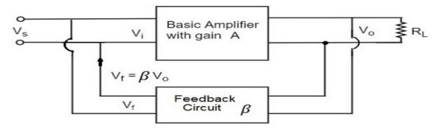
As the feedback circuit is connected in shunt with the output and the input as well, both the output impedance and the input impedance are decreased.
