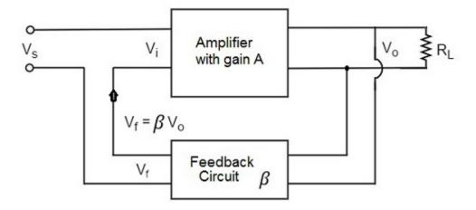
As the feedback circuit is connected in shunt with the output, the output impedance is decreased and due to the series connection with the input, the input impedance is increased.
