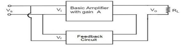
As the feedback circuit is connected in series with the output, the output impedance is increased and due to the parallel connection with the input, the input impedance is decreased.
